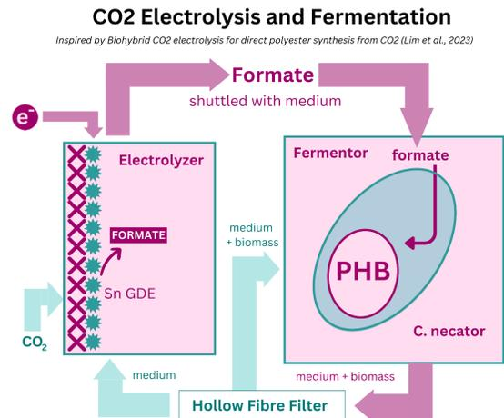
Figure 2. Biohybrid Electrolysis and Fermentation Chambers
